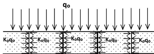
Fig. 4: The mechanics of geocells as load support systems
