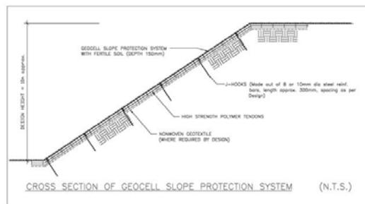
Fig. 8 Geocells with vegetation for slope protection
