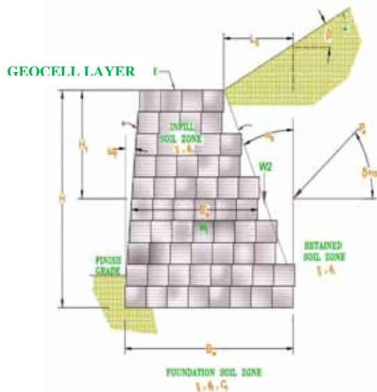
Fig. 5: Typical gravity wall of geocells
