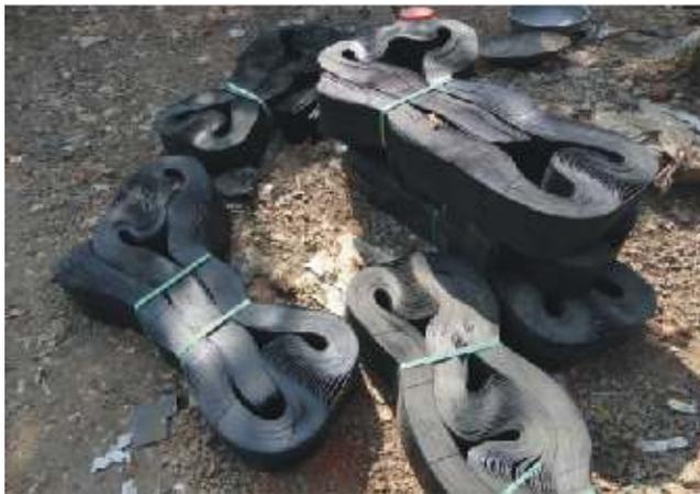
Fig1: Collapsed panel of StrataWeb
